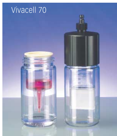
Vivacell 70 Centrifugation Pressure 70 ml* - 150 µl**
